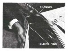
3. Remove the soft top from the pocket provided at rear of seats, holding the metal front section near the centre pins.
