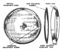
against the tension of the adjustment screw springs and turn it in an anti-clockwise direction until the heads of the screws can be disengaged through the slotted holes in the Light Unit rim. Do not disturb the screws when removing the Light Unit or the Lamp setting will be altered. Twist the back shell in an anti-clockwise direction and pull it off. The bulb can now be removed from the rear of the reflector.
