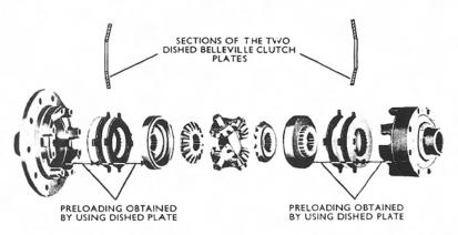
LOADING OF FRICTION CLUTCHES BY BELLEVILLE SPRING
