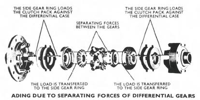
**3.** Cam Loading. The cam faces of the cross pins which engage vee slots in the differential case halves, impose a loading on the cross pins along the axis of the differential when torque is transmitted by the differential assembly. This re-action is transmitted to the side gear clutch rings through the abutment shoulders on the differential pinion mates.
