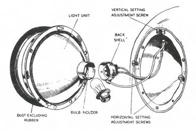
Position the Light Unit so that the heads of the adjusting screws protrude through the slotted holes in the flange, press the unit in and turn in a clockwise direction. Replace the rubber ring so that the thicker inner edge rests in the recess around the Light Unit rim.
