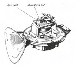
It is also possible that the performance of a horn may be upset by the fixing bolt working loose, or by some component near the horn being loose. If after carrying out the above examination the trouble is not rectified, the horn may need adjustment; but this should not be necessary until the horns have been in service for a long period.
