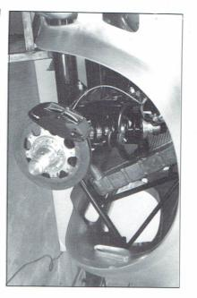
There are some areas we felt needed a little updating while keeping the look and feel of the car auther tic. The front suspension is an example of how a reproduction of an original can be made better using late model ball joints, bearings and seals. These upgrades will give you many miles of dependable service.
