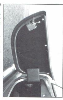
The detail seen here is the ¾" steel tube frame bonded to the outer fiberglass skin. The hinge assembly is a reproduction of the original design manufactured from heavier material and incorporating a bronze bushing for smooth operation. Even the latch is the same as the one used on the original.
